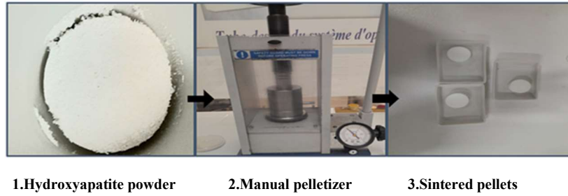
Figure 2. Preparation step for sintered samples at 1100°C for 3 hours.
